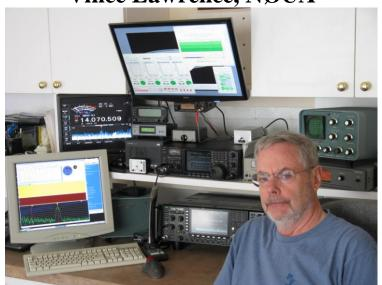
**HF Transceivers:** Icom IC-7700 (with external monitor), IC-756ProIII, IC-706MKIIG
